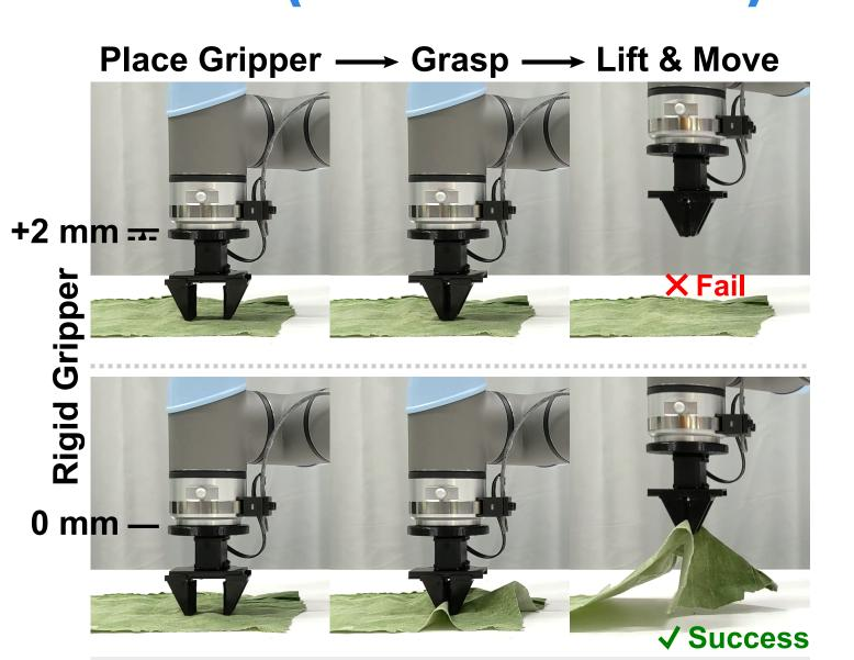
A rigid gripper's low compliance induces large normal forces under uncertainty in vertical positioning.
