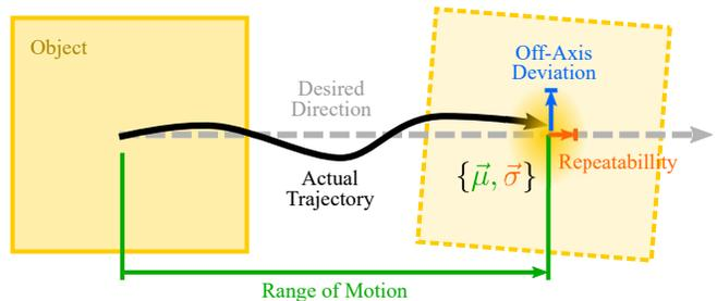
Fig. 2. We introduce three task-based performance metrics for in-hand manipulation. The *range of motion*, *repeatability*, and *off-axis deviation* measure the performance of a given motion primitive task.
