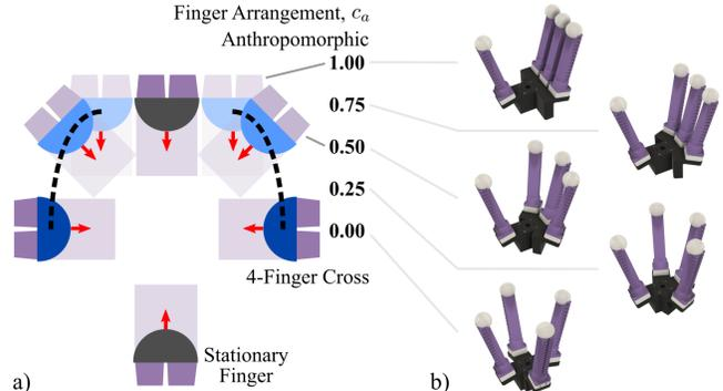
Fig. 1. In this study, we are interested in the effect of finger arrangement on in-hand manipulation capabilities. a) Based on the 2-DOF fingers from [14], we controlled the resting pose of two fingers in the hand along an ellipse to smoothly transition between “4 finger cross” and “anthropomorphic” arrangements. Using simulations and b) physical prototypes at five discrete finger arrangements, we explore the effect of finger arrangement on manipulation of a wide variety of objects.
