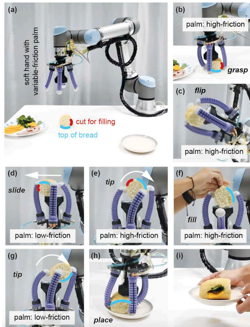
Figure 6.13: The actuated palm enables a real-world grasping and manipulation task: Helping a worker make a submarine sandwich.
